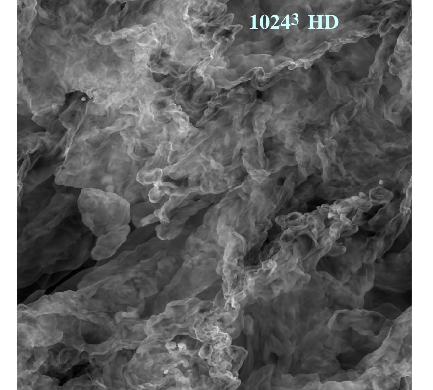
In HD the numerical **resolution** is crucial to capture the instabilities of postshock shear layers.
