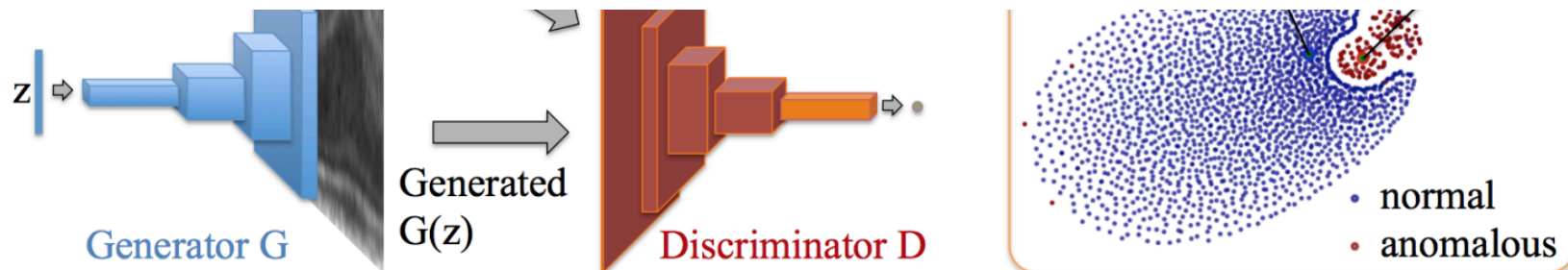
Fig. 2. (a) Deep convolutional generative adversarial network. (b) t-SNE embedding of normal (blue) and anomalous (red) images on the feature representation of the last convolution layer (orange in (a)) of the discriminator.
