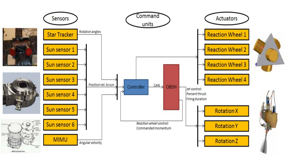
Fully redundant system, 3-axis stabilized,  $\Delta \phi < 0.05 deg$ ,  $\omega < 0.15 deg/s$
