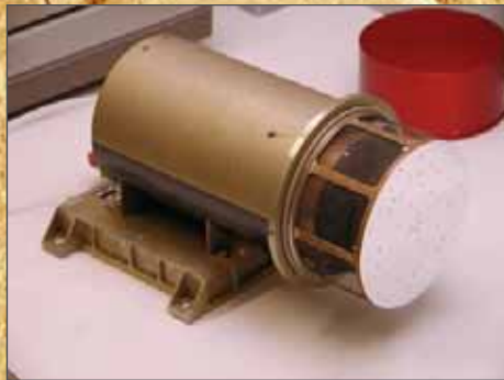
ASPERA: Energetic Neutral Atoms Analyser PI: M. Holstrom, IRF Kiruna (SE)
