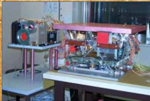
OMEGA: Visible and Infrared Mineralogical Mapping Spectrometer PI: J. P. Bibring, IAS Orsay (FR)
