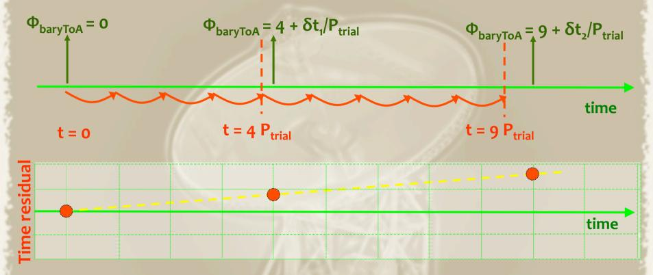
From a least square fit, one gets a P<sub>new</sub> allowing the rms residual to go closer to 0
