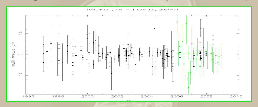
The quality of the timing solution is usually given in term of the root mean square **rms** of the residuals:
