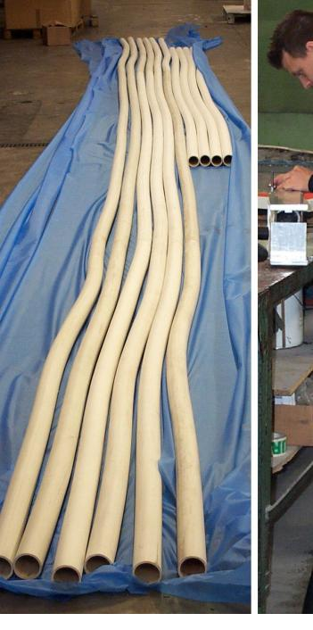
Rubber tubes at the factory of Hercorub. Light coloured rubber was not stable enough for bad weather sealing. Solved with inside tubes of stiff black rubber, which gives stiffness to the outside tubes. Stiff black rubber is from similar compound studying the Solar magnetic fields essential for but with added carbon for the stiffness.
