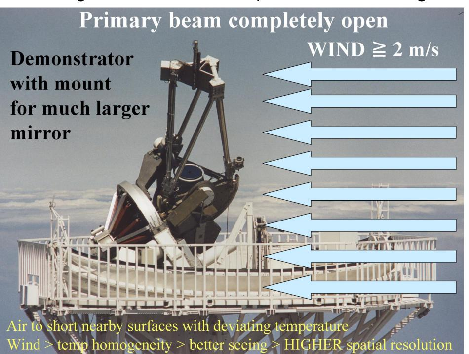
Solution for high resolution observations telescope: Open structure and completely open-foldable dome of which all parts remain relatively cool in sunshine, only few degrees increase in temperature. Air has no time to take over different temperatures from mount and dome. The DOT, successful demonstrator.
