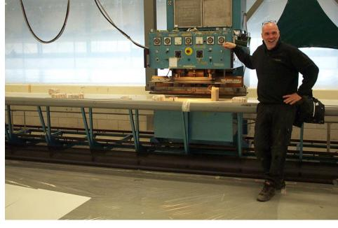
Production in the large factory hall of Poly-Ned of the light coloured textile membranes from many strips to form the stable saddle shape.
