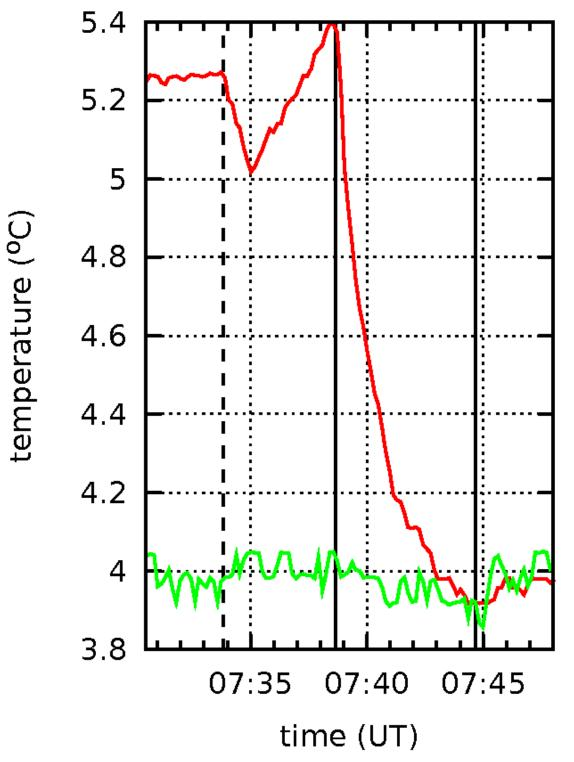
After opening, the air temperature inside the dome is very fast equal to the outside air temperature. Left side registration of whole morning, right side detail of opening.
