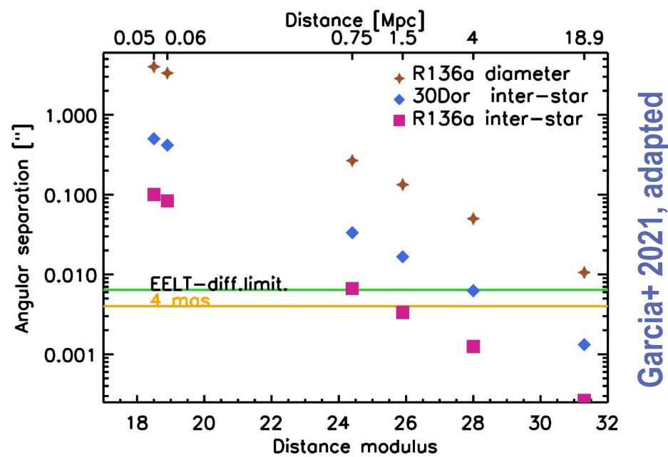
The 4 miliarcsecond (mas) scale fully samples the Airy disk at 1µm. HARMONI will break down R136a-like clusters as far as the outer Local Group, enabling studying the impact of environment (star-formation rate, metallicity) on the upperend of the initial mass function, thus setting observational constraints to the theories of massive star formation.
