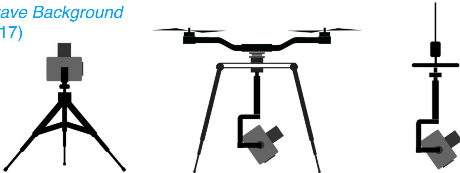
Fig. 1. Three different configurations for POLOCALC (starting from the left): 1) from a ground tripod 2) from a flying drone and 3) from a high-altitude balloon.
