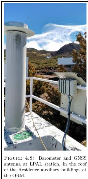
FIGURE 4.8: Barometer and GNSS antenna at LPAL station, in the roof of the Residence auxiliary buildings at the ORM.
