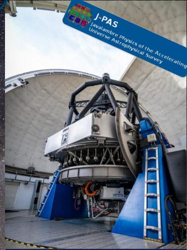
JST250 Ritchey-Chrétien plus Field Corrector Diameter = 2,55 m FoV = 3 deg \emptyset F/3,5 M2 hexapod
