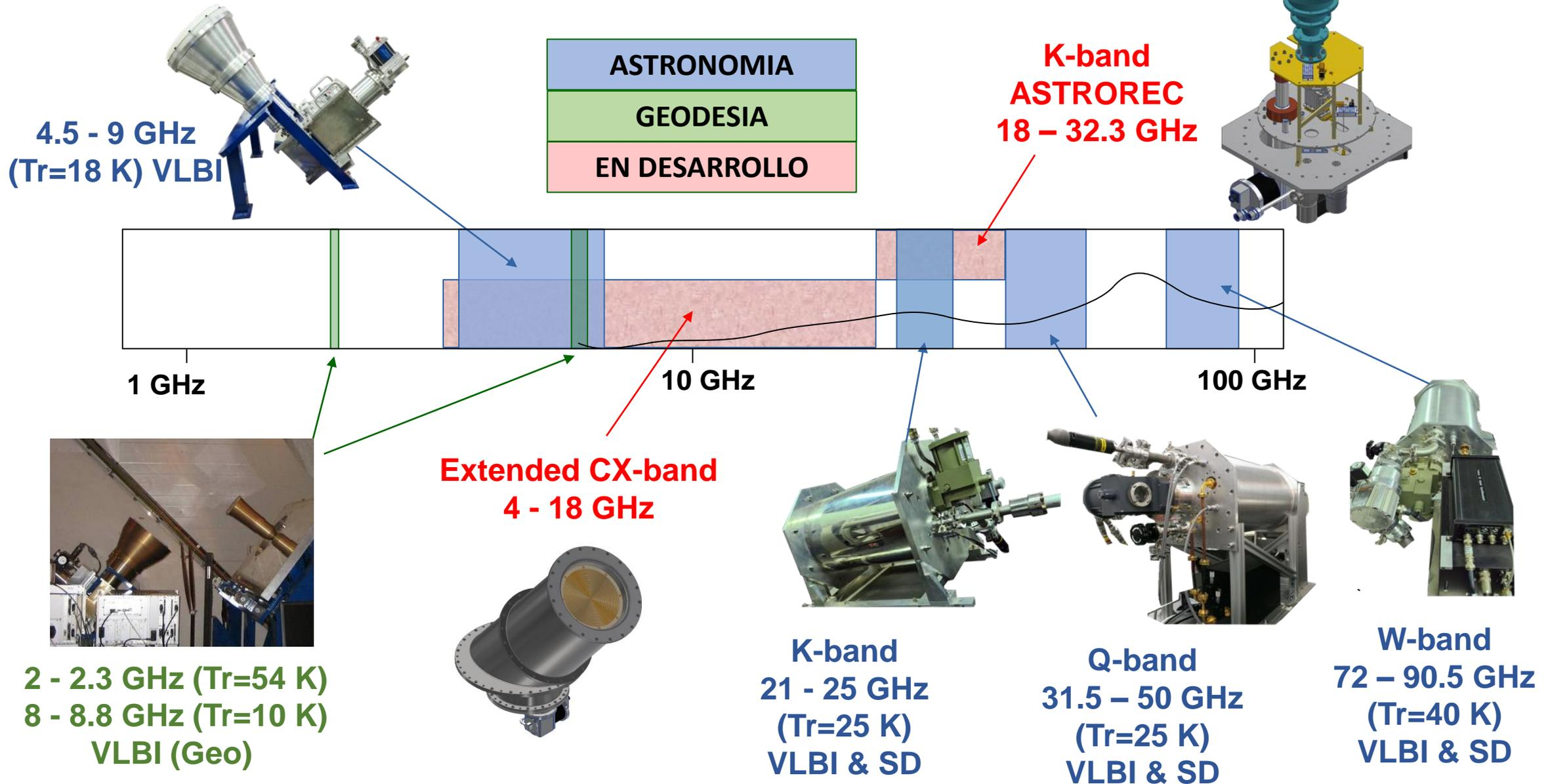
Cryogenic systems are usually stable and **low-maintenance** in the long term
