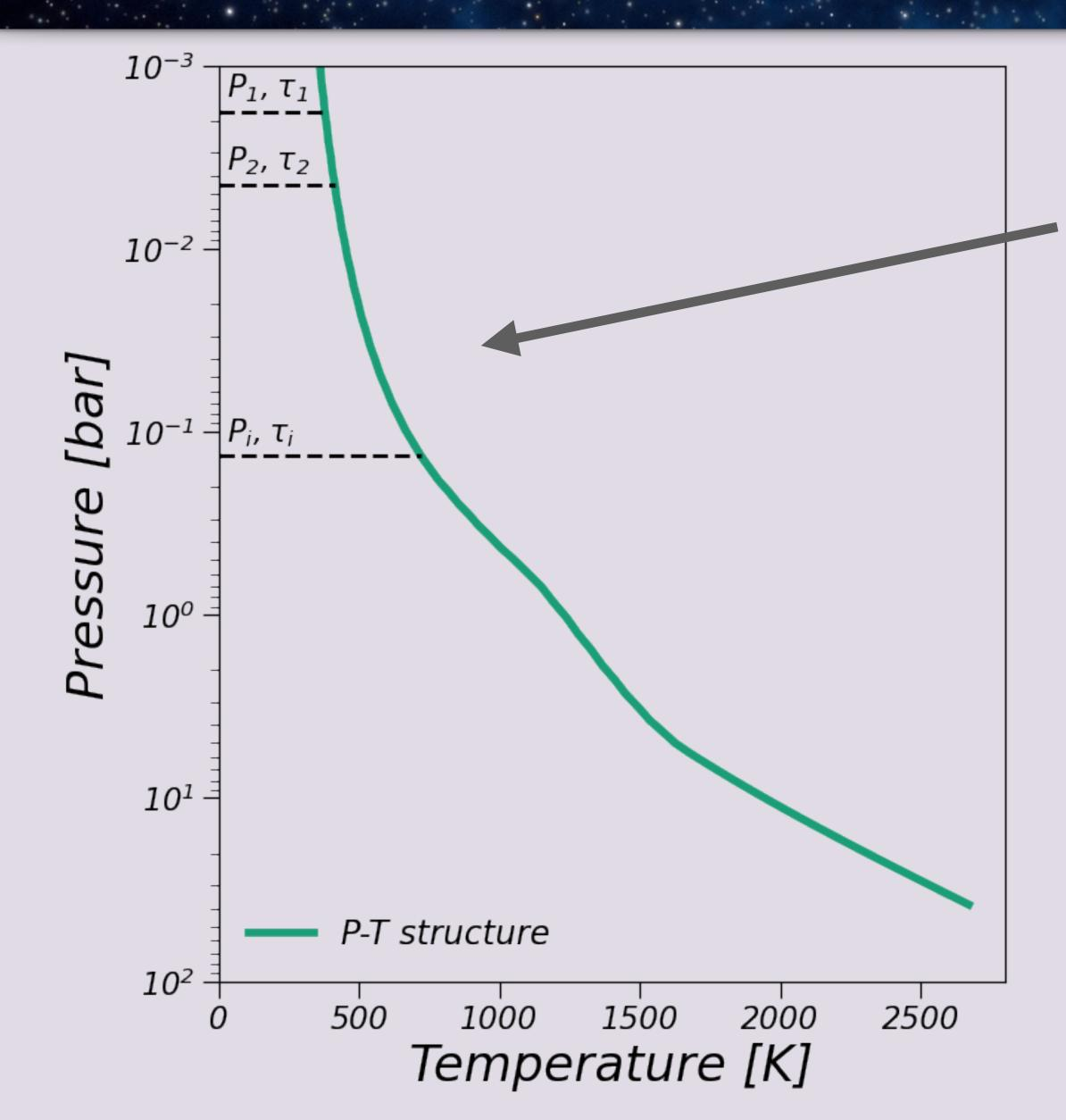
Vertical column of gas split into a grid of model levels defined in pressure, altitude or optical depth
