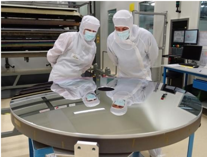
Al coating for the OAJ observatory mirror diameter 1,25m weight 320kg
