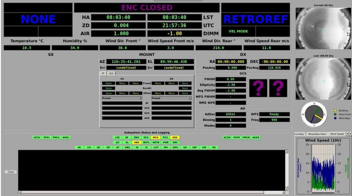
Figure 9. The FACSUM at the LBTO. The basic telescope information (dome open/close, elevation, RA, authorized instruments, etc), site environments (wind speed, seeing, humidity, and so on), TCS subsystems information, the AO system and its ASM information, are shown.
