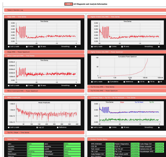
Figure 5. FLAO diagnostic and analysis information. The wavefront RMS, ASM commands RMS, Tip-Tilt and other parameters can be shown in different time scale. The low level system status with color can help the AO operator to notices the errors.
