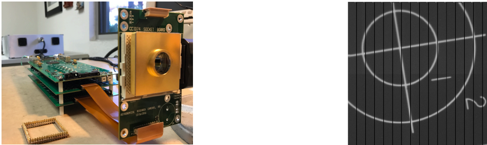
Figure 9: Left: ARC readout electronics prototype. Right: Early test image from VCAM using an engineering grade CCD74 (the vertical black lines are deliberate to allow easier identification of individual video channels)
