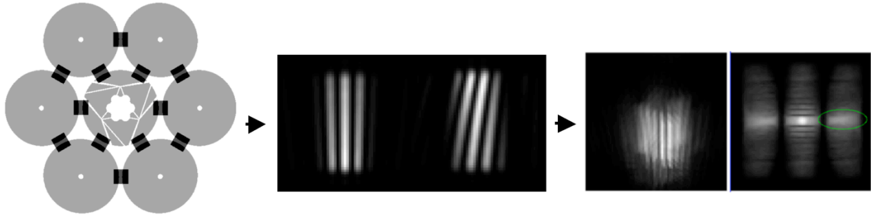
Figure 3: Left: The GMT pupil overlaid with 1.5 m square apertures at the segment boundaries. Center: Simulated fringes from one subaperture showing in phase (left) and a 10 micron phase shift (right). The dispersion direction is vertical. Right: A simulated dispersed fringe image and its FFT. The vertical position of the circled peak is a function of the tilt of the fringes and thus a measure of the piston error.
