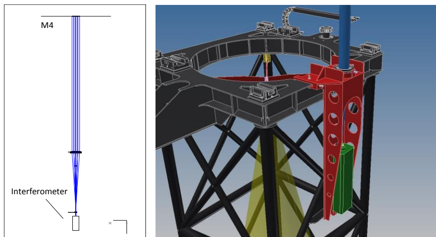
Figure 7: SAI test setup optical and mechanical designs.
