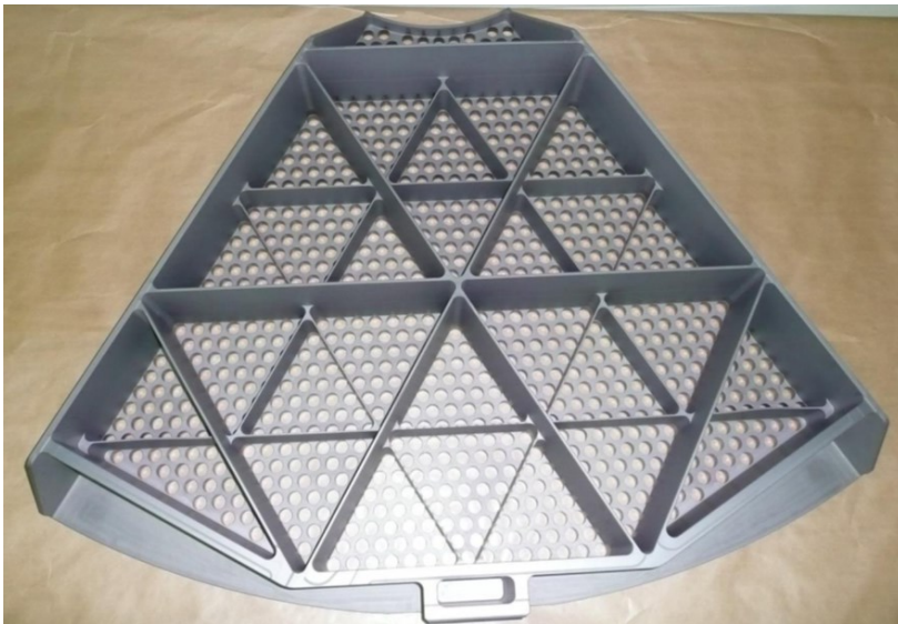
Figure 8: second segment manufactured. The most left and right ribs are bent by 2 millimeters.
