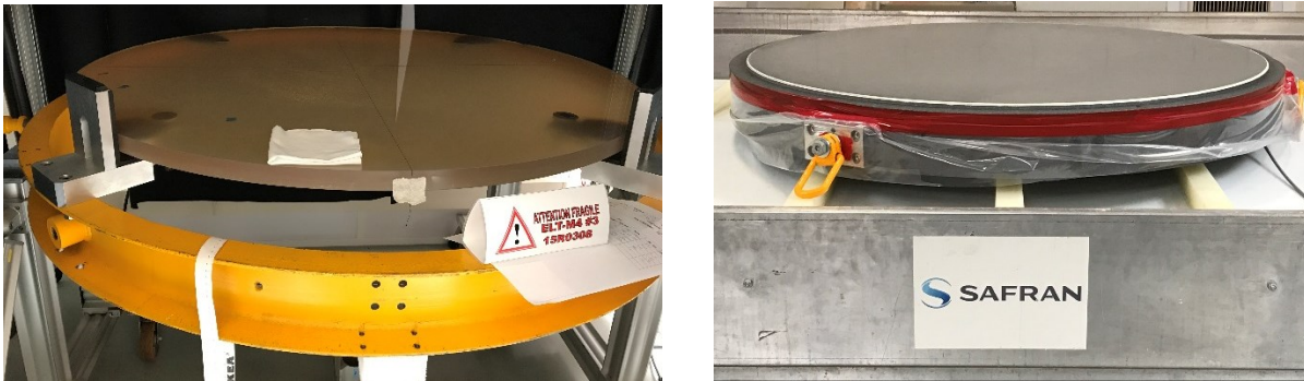
Figure 11: Shells under manufacturing: on the left during measurement inspection of the optical face. On the right at the start of the polishing of the back surface. The shell has already a thickness of 2 mm.
