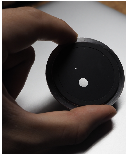
Figure 3. SCC modified Lyot stop. The classical stop is the large hole. The SCC reference hole is the small hole.
