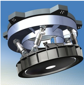
Figure 1: ELT's deformable mirror M4 (credits ESO).
