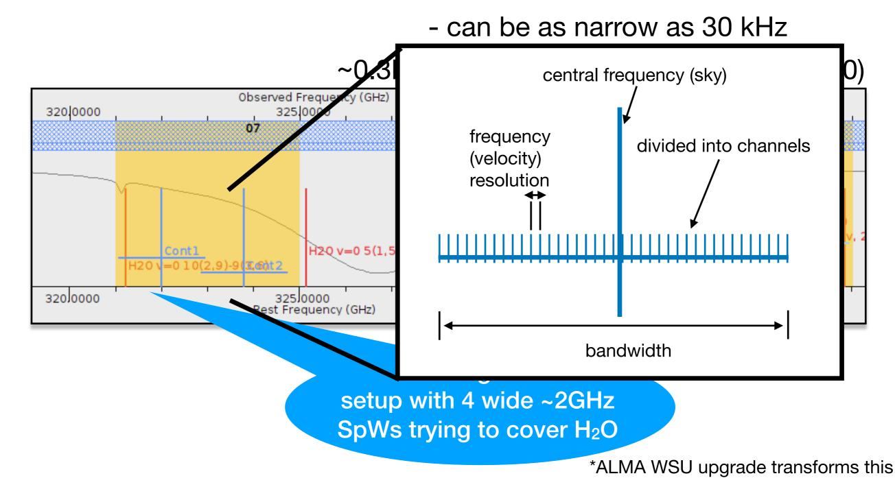
• Four configurable basebands - 58 MHz to ~2GHz spectral windows
