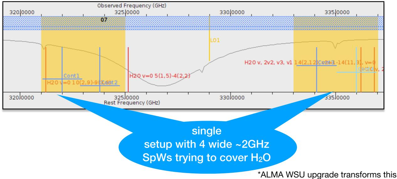
• Four configurable basebands - 58 MHz to ~2GHz spectral windows
