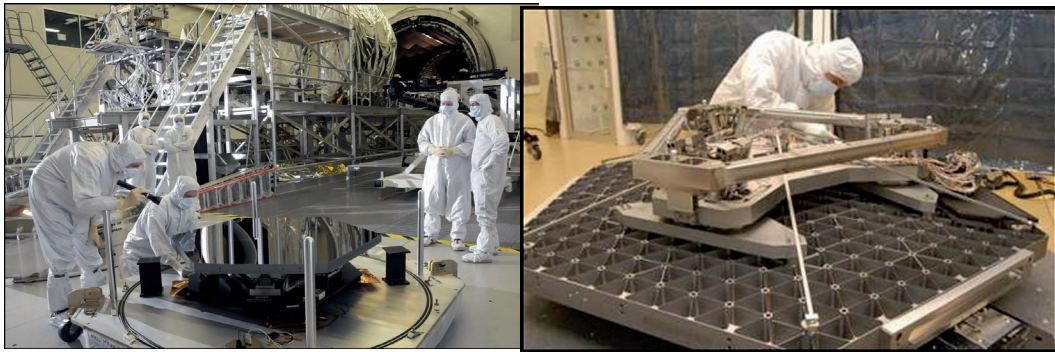
Figure 8. A primary mirror segment entering cryogenic testing (left), mechanized segment mount assembly provides 6 DOF and radius of curvature adjustment (right).
