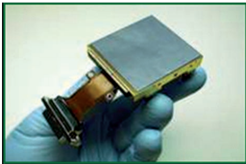
Figure 16. Left -- A Teledyne H2RG 4 Mpixel sensor chip array; Right -- noise performance of this technology (green cross) compared to that of 0.07 Mpixel InSb sensors used on the Spitzer space telescope (red dot). The lines shown are the original (circa 1999) requirement and goal for background limited performance (BLIP) for the JWST (then called NGST).
