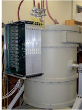
Figure 9. AzTEC cryostat and readout electronics.
