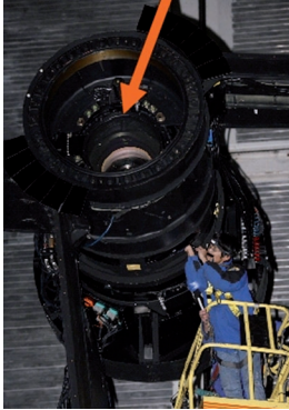
Fig. 13. Prime focus corrector for FMOS
