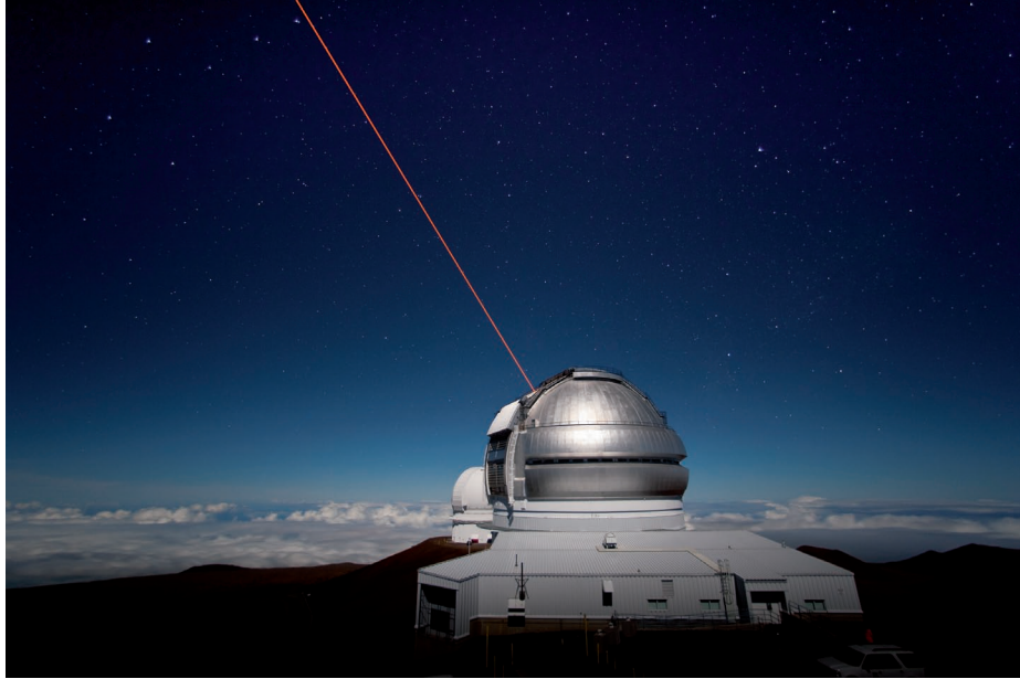
Figure 1. View of the Gemini North telescope with its 12-Watt solid-state laser beam propagating for laser guide star adaptive optics observations.
